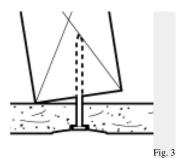
Cause: Framing members have not been properly squared with plates, presenting angular nailing surface (Fig. 3). When panels are applied, there is danger of puncturing paper with fastener heads or of reverse twisting of member as it dries out, with consequent loosening of board and probable
