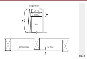
Cause: Due to misaligned top plate and stud, hammering at points "X" (Fig. 2) as panels are applied on both sides of partition will probably result in nail heads puncturing paper or cracking board. Framing members more than 1/4" out of alignment with adjacent members makes it difficult to bring panels into firm contact with all nailing surfaces.
