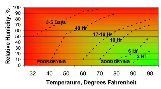
**Graph Reference** – The color-coded graph provides an easy-to-interpret map of joint compound drying time ranges based on the relative humidity and temperature conditions present on a job. To estimate joint compound drying time, simply select and cross-reference a temperature and relative humidity range to determine approximate drying time per coat (1/16 inch nominal).
